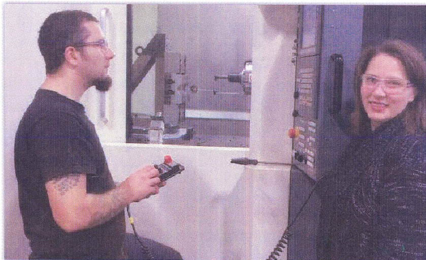
Kimberly Smith, president and general manager, and operator Nick Panza with the Kitamura HX630iTGA 630-mm HMC machining a 2" (51-mm) PLIDCO Split+Sleeve fitting for the pipeline and repair industry.
